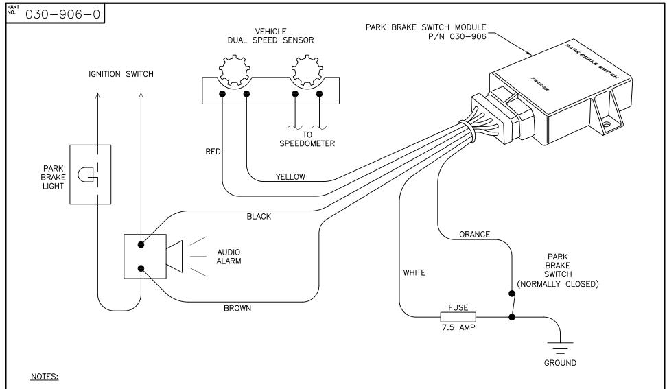
1. PART NUMBER DETERMINED BY APPLICATION: 030-906: NEGATIVE GROUND 12 VOLT. 030-906-1: NEGATIVE GROUND 24 VOLT.
